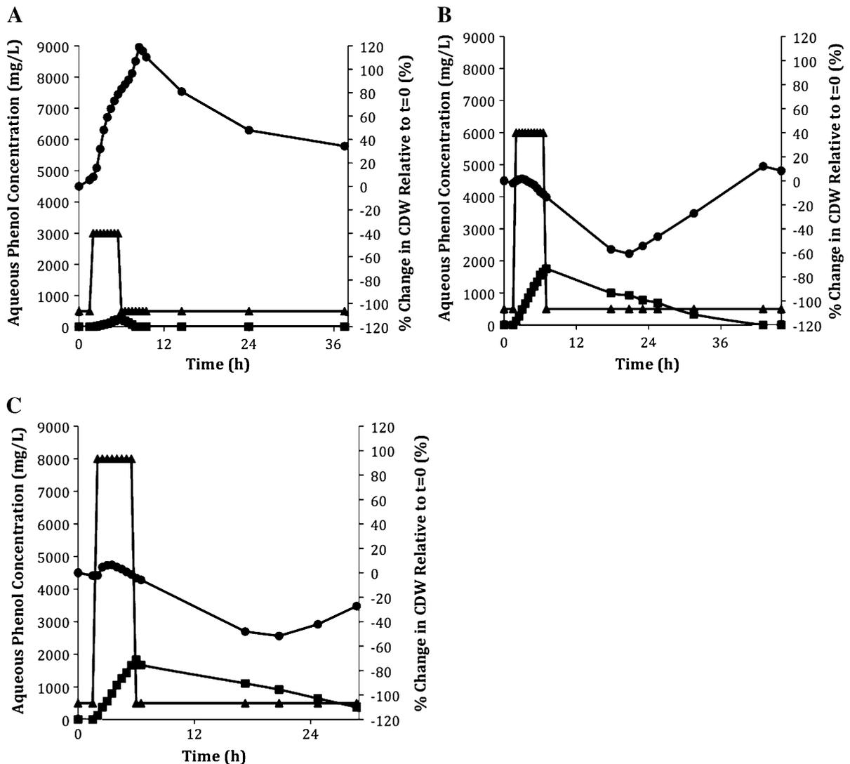
**Fig. 2** Single phase continuous operation with 4 h phenol step changes of varying magnitude (**a**: 3,000 mg/l, **b**: 6,000 mg/l, **c**: 8,000 mg/l). Filled circle are the percentage change in
