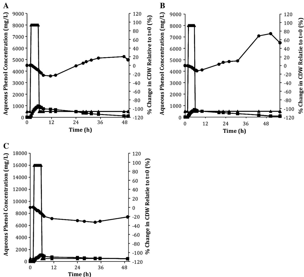
**Fig. 3** TPPB operation with 4 h phenol step changes of varying magnitude (a: 8,000 mg/l, 5 % (w/v) polymer, b: 8,000 mg/l, 10 % (w/v) polymer, c: 16,000 mg/l, 10 % (w/v) polymer).
