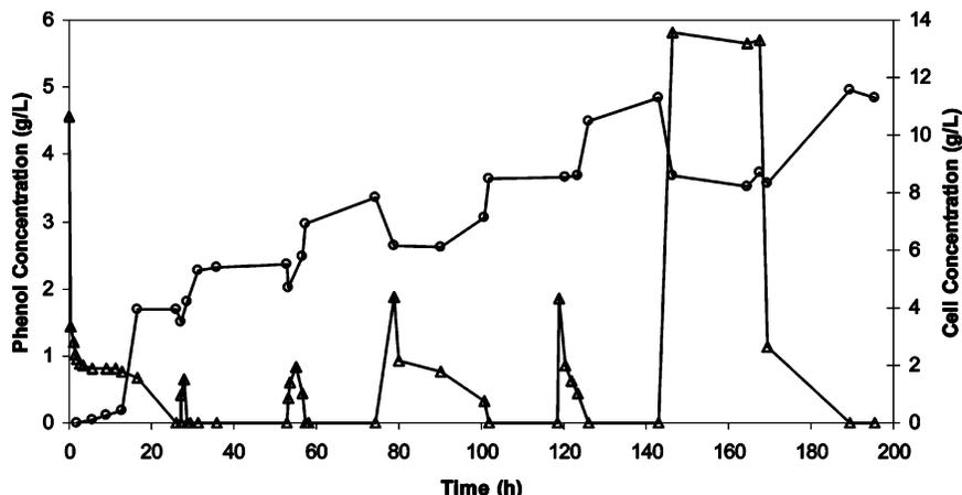
**Figure 5.** Batch fermentation of phenol followed by two bead replacements, two concentrated phenol spikes, and a final validation of the need for polymers in a TPPB. The triangles represent phenol concentration, and the circles represent cell concentration.
