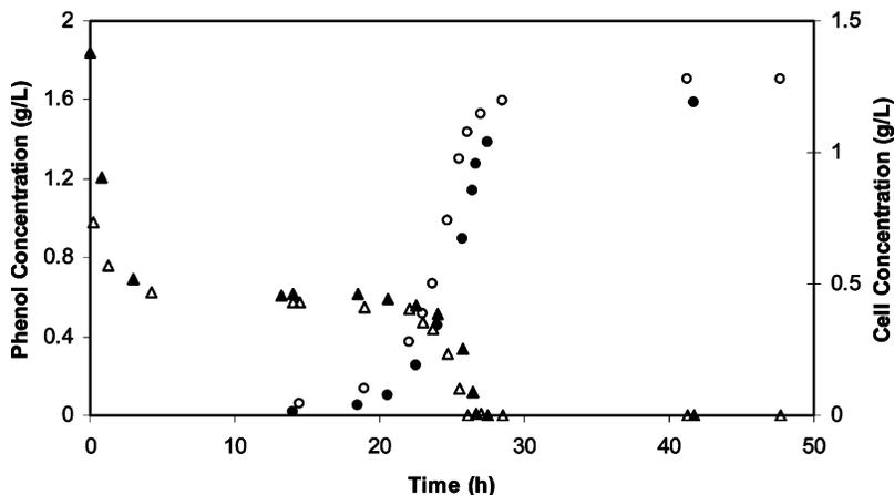
**Figure 3.** Batch fermentation with Hytrel polymer beads at an initial phenol concentration of 1840 mg/L. The open triangles and circles represent phenol and cell concentrations for fresh beads, respectively, and the closed symbols are for reused Hytrel beads.
