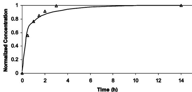
**Figure 2.** Absorption of phenol by Hytrel polymer beads comparing normalized concentration of phenol absorbed vs time. The experimental data are shown by the symbols, and the line represents the best fit, using the method of least squares, corresponding to a diffusivity coefficient of  $1.54 \times 10^{-7} \text{ cm}^2/\text{s}$ .
