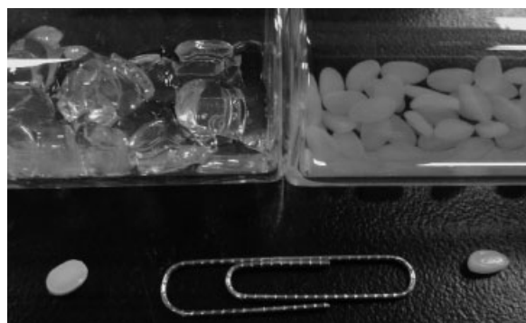
Figure 2. Photograph comparing swelling behavior in different grades of Hytrel® when exposed to indene: 3548 swelling and cracking on left, 8206 unaffected on right. Unexposed beads in foreground for comparison with paper clip for scale.
