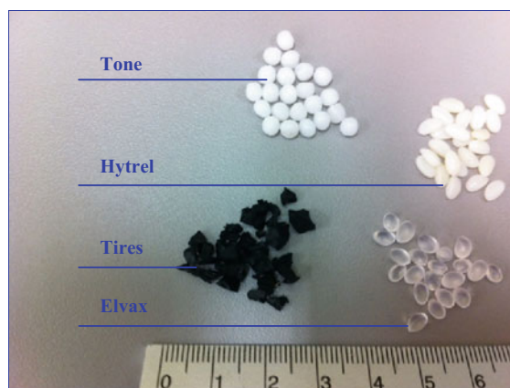
Fig. 1 Tires and commercial polymers in the form utilized in experiments with TPPBs (scale bar in cm)
